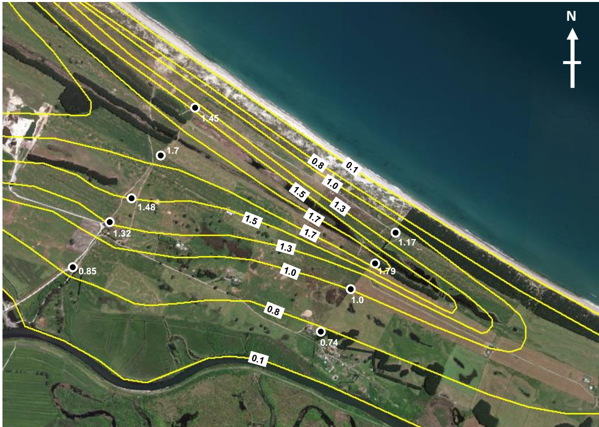
Figure C1 – Map showing the creation of median groundwater contours in the Te Tumu urban growth area.
